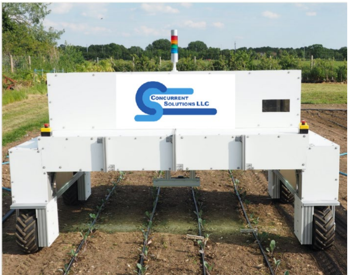
Figure 1 Prototype robotic platform specially designed, developed and built for the eyeSpot project by Concurrent Solutions llc in the USA. The platform was designed to treat four rows of vegetables planted in beds of two metres width. The platform is shown at Sonning Farm in July 2019 with four rows of cabbages (50 cm between rows; 30 cm between plants in rows.) The black tapes along each row are the drip irrigation system. The platform was demonstrated to growers and others in July 2019 at an AHDB Open Day, which was organised to disseminate and demonstrate the results of the eyeSpot project.
